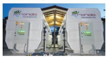
The Miracell wastewater treatment system has a modular design, with units that can be configured to service small to mid-sized communities between 50 and 20,000 people or businesses with water treatment needs of 2,600 gal/day - 1,058,200 gal/day. It is one of the most flexible and expandable systems on the market today, where modules can be easily added or moved to accommodate changes in demand. The system is certified to meet or exceed strict EU environmental discharge and irrigation standards.
